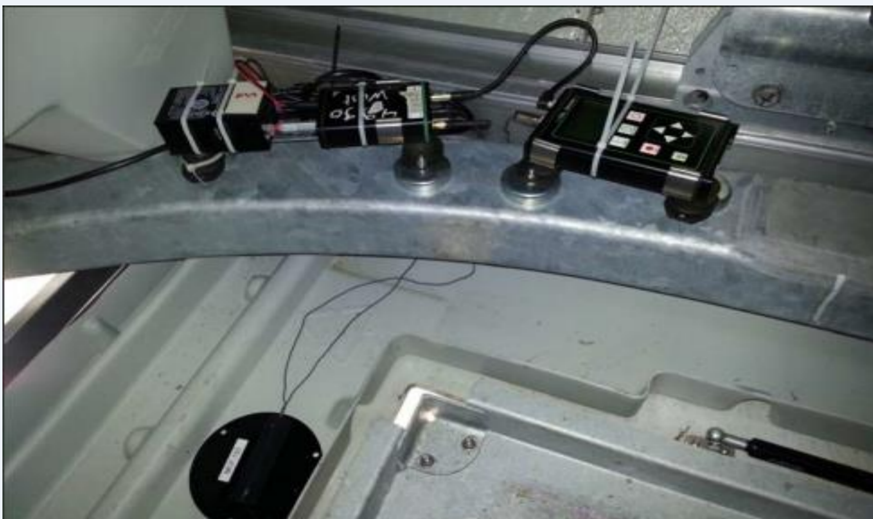
Figure 1. Ultrasonic detector „batcorder 2.0“ with “wind turbine extension” in a wind turbine nacelle. The microphone in the bottom left of the picture is orientated towards the bottom of the nacelle.
