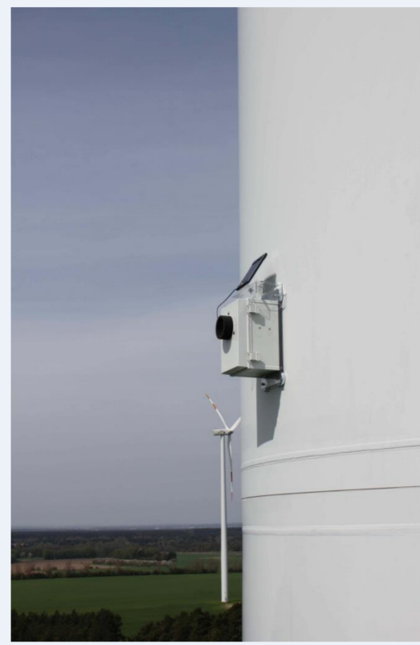
Figure 2. Installation of ultrasonic detector at wind turbine at 55 m.
